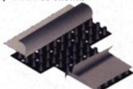
Fold back fabric and secure with tape to prevent soil intrusion
