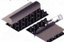
Interlock the dimples to connect the strip drains as shown.
