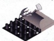
Wrap fabric around the end and secure with tape.
