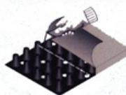
Wrap fabric around the end and secure with tape.
