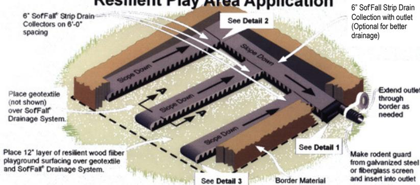
Sof'Fall Drainage is placed beneath the geotextile fabric, and provides for rapid drainage of water from the playground site. For full details and specifications, please visit [www.sof-solutions.com](http://www.sof-solutions.com).
